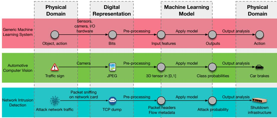
Figure 2. **System’s attack surface.** The generic model (top row) is illustrated with two example scenarios (middle and bottom rows): a computer vision model used by an automotive system to recognize traffic signs on the road and a network intrusion detection system.
