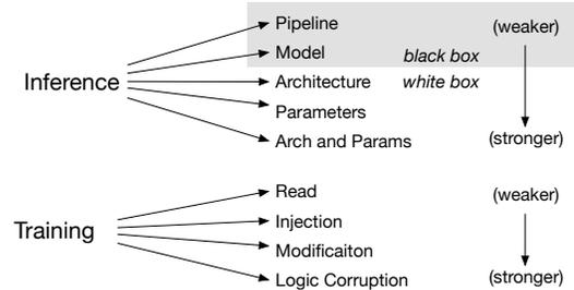
Figure 3. **Adversarial Capabilities.** Adversaries attack ML systems at inference time by exploiting model internal information (white box) or probing the system to infer system vulnerabilities (black box). Adversaries use read or write access to the training data to mimic or corrupt the model.
