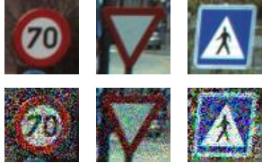
Figure 29: Speed planning attack images. Top row shows original images u , bottom row shows attack images u' which satisfy u' = u + \delta , \|\delta\|_\infty \leq 0.32 . We note that images in this setting are represented by a 3 \times 56 \times 56 tensor, with pixel values normalized from [0, 1] . Images may look worse than they appear due to artifacts from stretching the attack perturbations since input images are of low resolution. All attacks were found using AllZeroRowCol in the ReLU setting.
